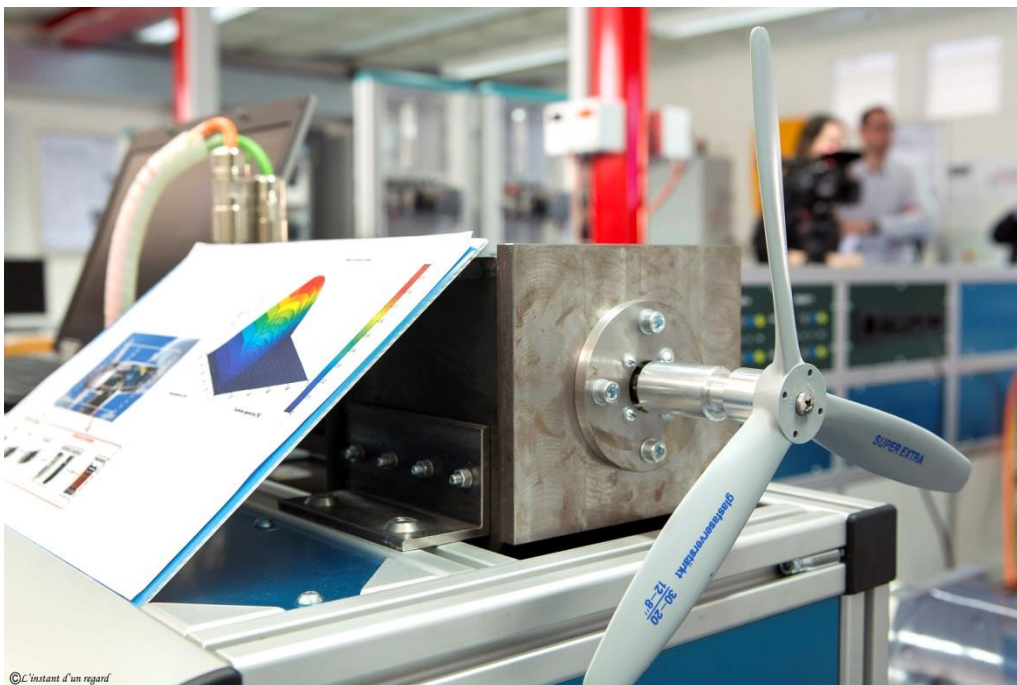
Fig. 4 – Detail of the reduced-scale model of a wind turbine
