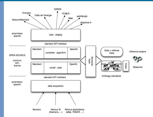
The many different **energy management information systems for buildings** have each been developed for a specific purpose. This means that the professionals in this field frequently have to use several solutions which are often partially redundant
