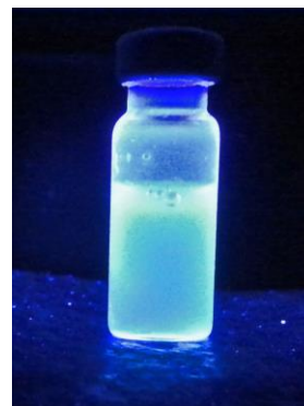
HPLC-vial under UV light after rehydration with arsenic-containing sample
