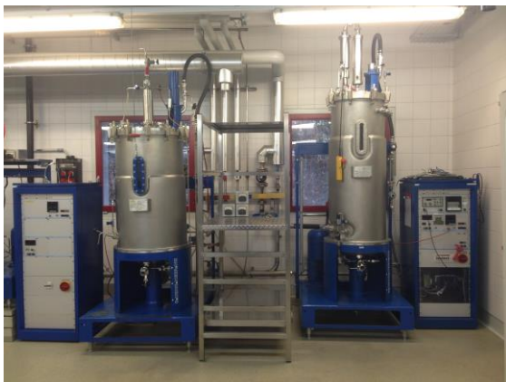
Two 300 L bioreactors are available for the scale-up of the production process.
