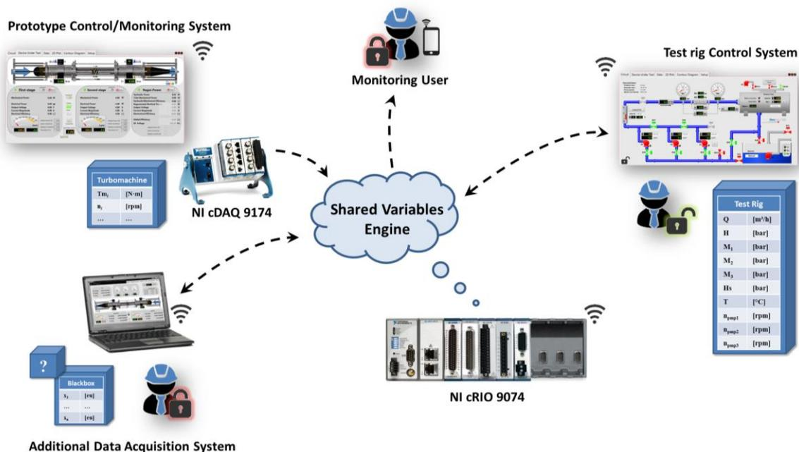
Figure 2. Multi-user control system architecture of the test rig.
