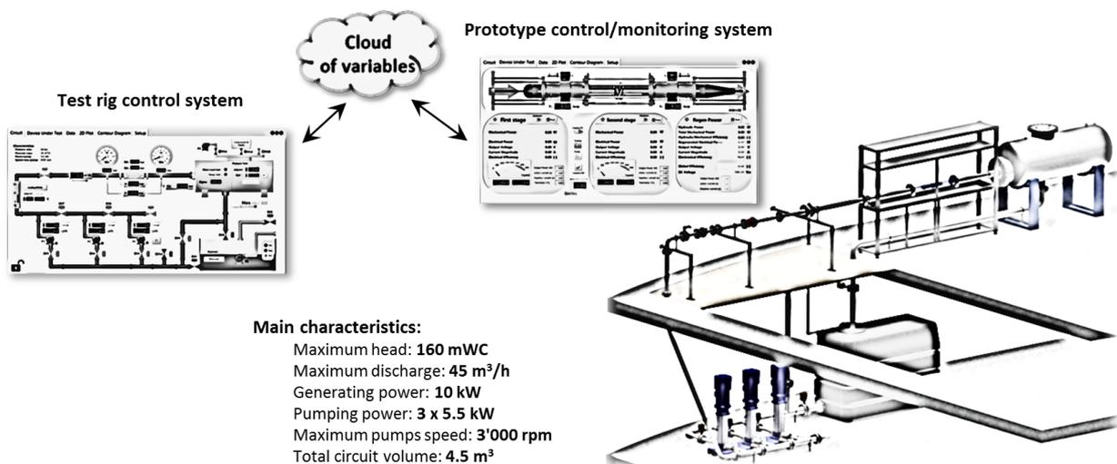
Figure 1. New hydraulic test-rig of the HES-SO Valais/Wallis – Sion, Switzerland, Hasmatuchi et al. 2014.
