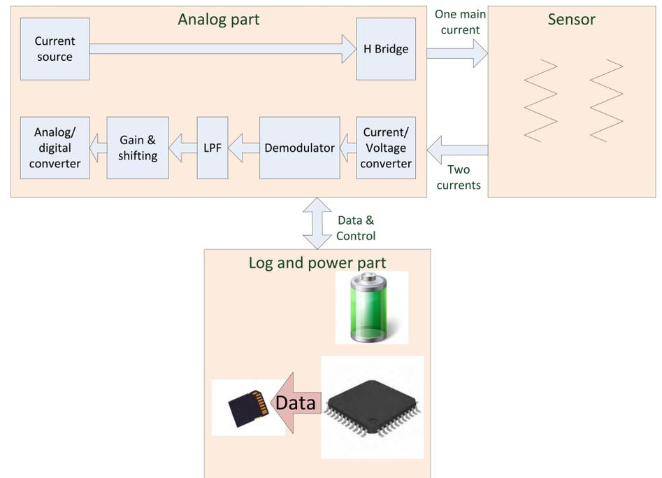
The figure above shows a block diagram of the sensing acquisition, processing and recording / read-out electronics.
