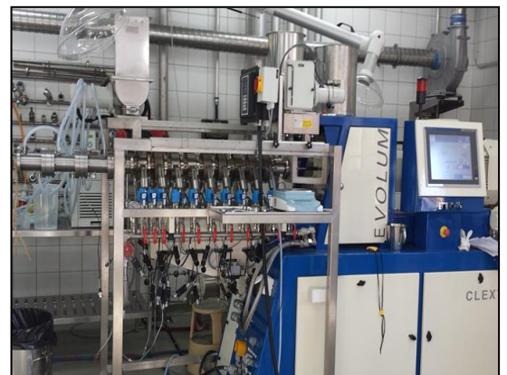
Extruder Evolum 25 (Clextal) used in pea protein fibrillation
