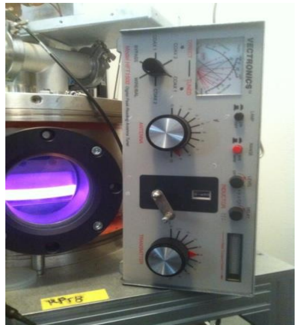
Capacitively coupled, low pressure flat plate reactor
