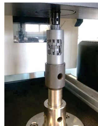
Setup made to deform the 10 wires of the stair actuator with the tensile machine.
