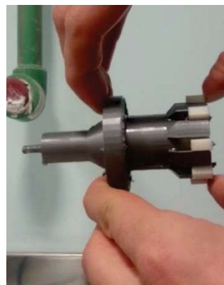
Screenshots of a video showing the fluid actuator functioning without the Shape Memory Alloy wires. The rod goes outside when pushing the white part
